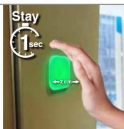
The IR sensor activated, and the door will open automatically.
